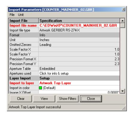
Select the *Show Filters* option so that the unwanted items can be filtered off as shown in figure below.
