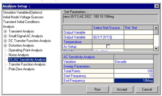
This analysis helps to calculate sensitivity of an output variable (voltage and current) with respect to all circuit variables, including model parameters.
