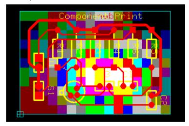
7. Labels may be placed to display the field intensity at various points on the board. For this select the tool Set/ Delete labels and click on the board at required locations. Label gets tagged to the cursor. Now drag the mouse to place the label at proper place.
