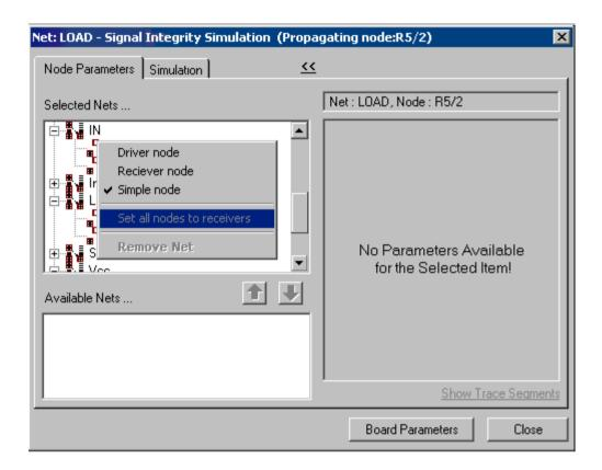
5. The electrical properties of the trace will influence the signal as it passes through it and this is shown in the respective columns. The Trace Segment parameters of the driver node may be viewed by clicking on **Show Trace Segments**.
