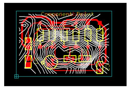
6. Color mapping on the board and may be viewed by switching on the option Colored board under View → Analysis Results → Colored Board. The analysis result is obtained. The Maximum and minimum field intensity locations can be observed.
