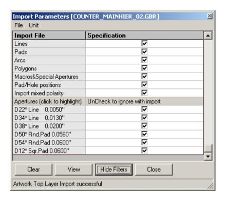
Uncheck the Imported elements items, which are not required. Since here the artwork top layer is imported, the board items are excluded by unchecking D22\* line 0.0050".
