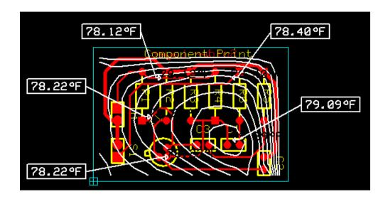
5. After adding these nets you may execute the analysis directly. For this right click and select the tool **Execute Analysis**. The result is displayed in the form of isolines.
