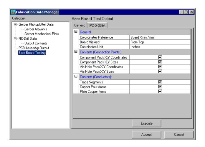
The output for Bare Board Testing is obtained as a text file.
