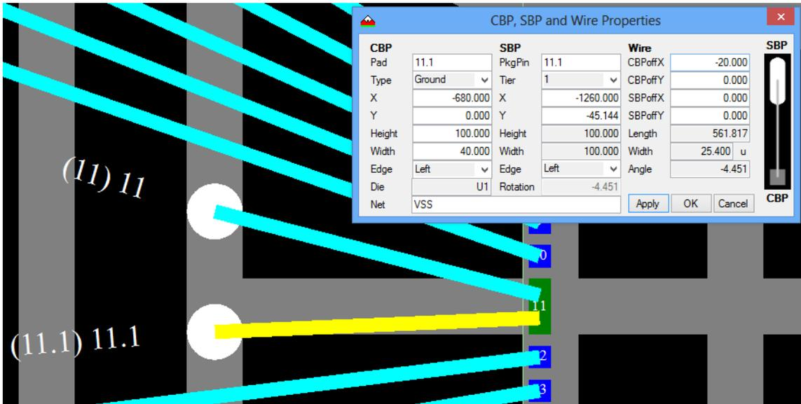
The result of this is pad 11 now has two wires attached to it. (11) 11 and (11.1) 11.1. Since this is in a pad ring you might reduce the Pad to Pad DRC rule for that tier for a tighter design. This depends on the bonding house and what their wire to wire rules are.
