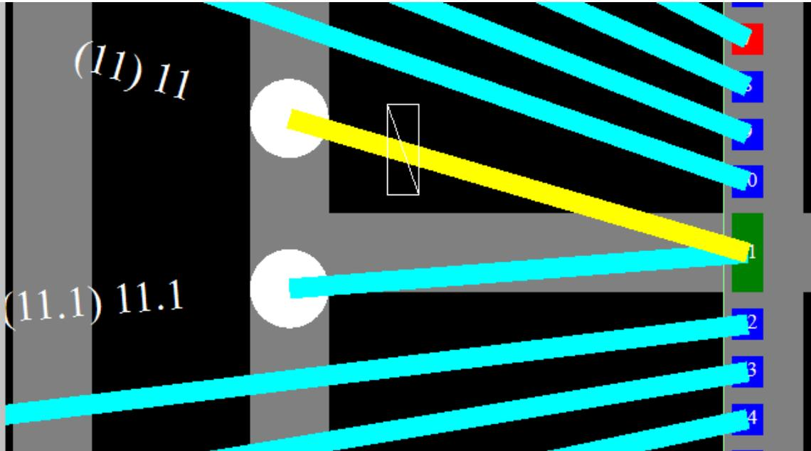
Open the Pad Properties dialog box and the selected wire information will be displayed. In this case I entered 20 into the CBPoffX box and pressed enter to accept the value. Then clicked on the Apply button. As you can see the CBP wire attach point has moved 20 microns to the right. (upward in this case). *Remember the offsets are based on the view at the right of the dialog box.*
