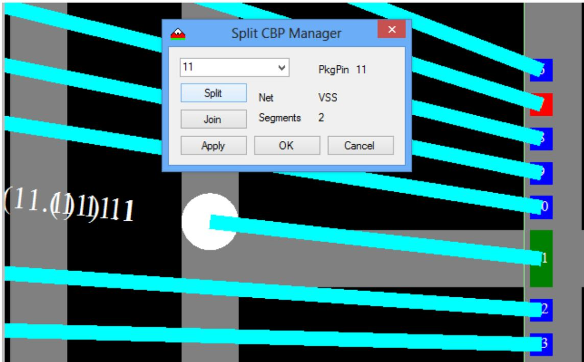
After fanout has been executed again you will see that the 2 segments have been fanned out based on the DRC rules set in the Tiers Properties dialog box. Now the 2 CBP attach points have to be separated.
