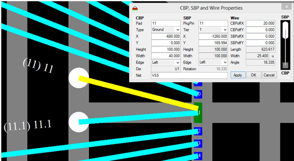
Next select the second segment and set the CBPoffX to -20 and click the Apply button and the CBP wire attach point is moved 20 microns to the left (down in this case).
